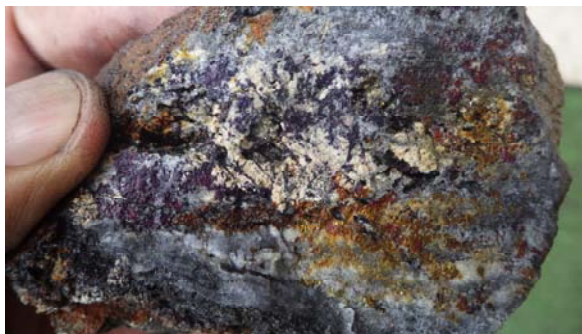
Photo 5: R02000489 – 1.4% Cu, 0.07 g/t Au, 0.19 % Zn Quartz vein with Cpy and Bn. Disseminated Cpy
