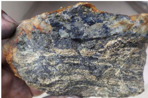
Photo 3: R02000495 – 2.07 % Cu, 0.24 g/t Au, 0.63 % Zn Quartz and magnetite veins, disseminated Cpy
