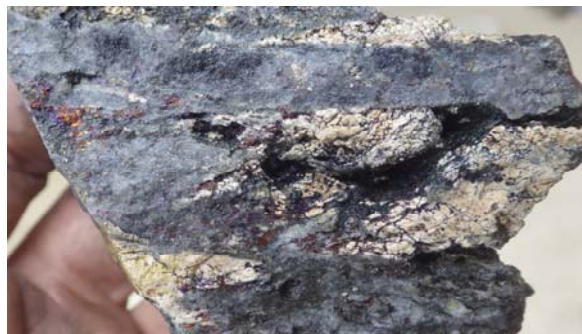
Photo 6: R02000493 – 1.25 % Cu, 0.21 g/t Au Quartz and magnetite veins, disseminated Bn, Cpy and Cc
