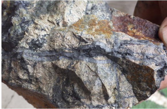
Photo 1: R02000494 – 2.23% Cu, 0.21 g/t Au, > 1% Zn. Quartz and magnetite veins with disseminated bornite (Bn), chalcopyrite (Cpy) & Chalcocite (Cc)
