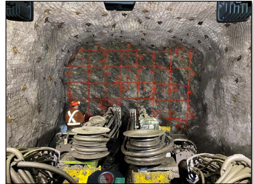
Jumbo preparing to drill on a LFZ development heading
