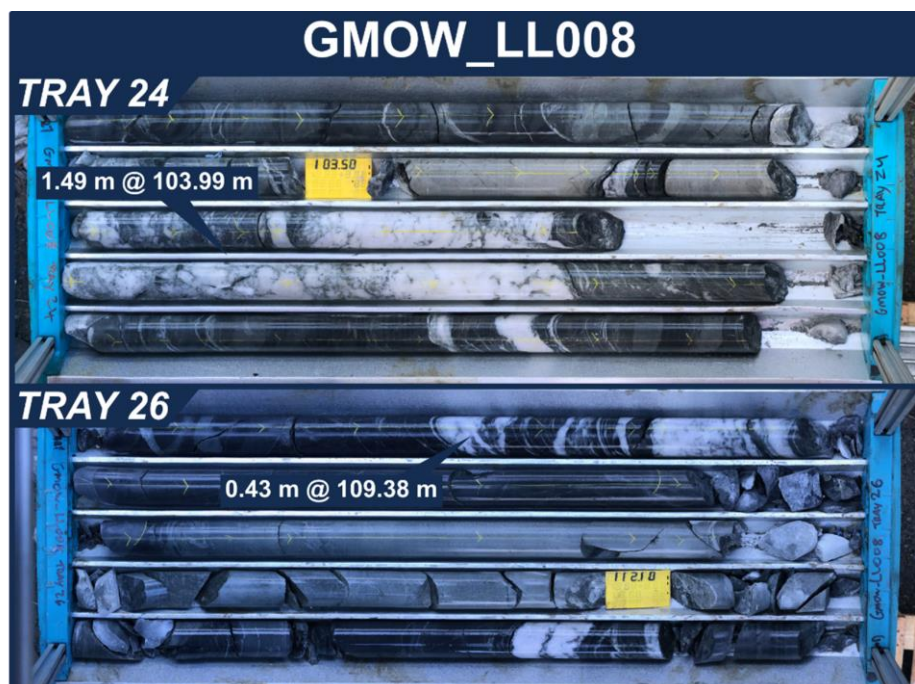
Figure 2: Core photos of key intercepts in GMOW_LL008, including a significant 1.49 m intersection of the target lode structure.
