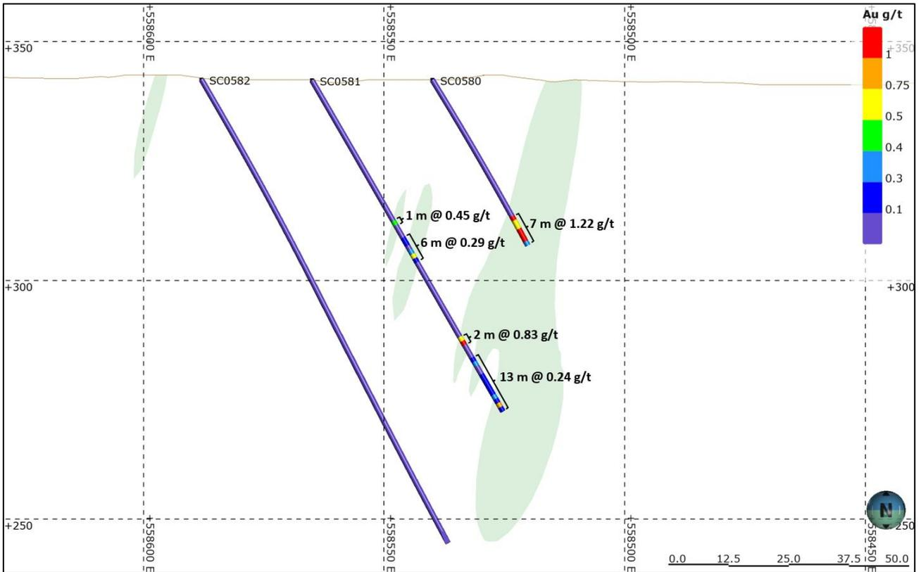
**Figure 4:** Cross section 1 looking south at Zone B North showing new drill hole traces and samples relative to a conceptual interpretation of the mineralisation.
