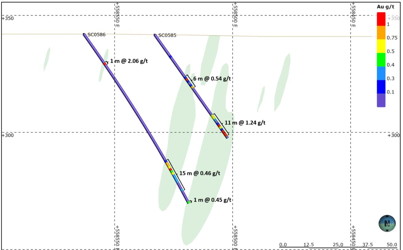
**Figure 5:** Cross section 2 looking south at Zone B North showing new drill hole traces and samples relative to a conceptual interpretation of the mineralisation.
