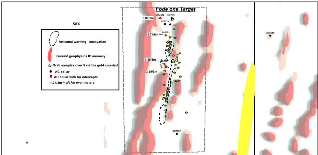
**Figure 2:** Fode 1 target showing the AC collars relative to the ground geophysics IP anomaly. The red dots show collars with gold intercepts in Table 1.
