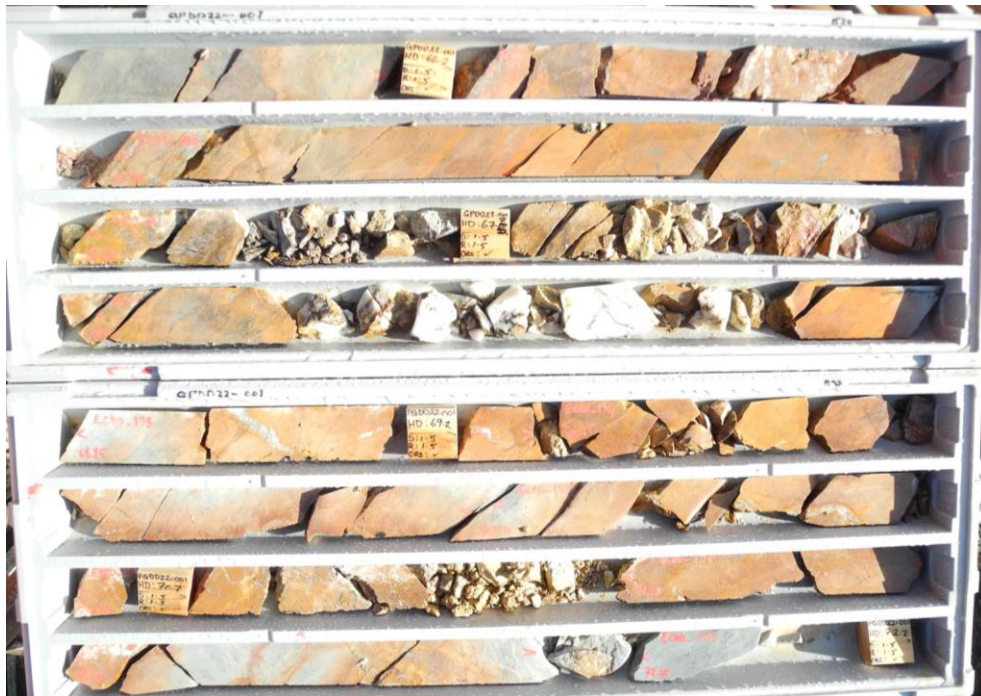
Figure 3. Homeward Bound diamond drill core samples showing mineralised laminated quartz vein and enhanced weathering around the structure
