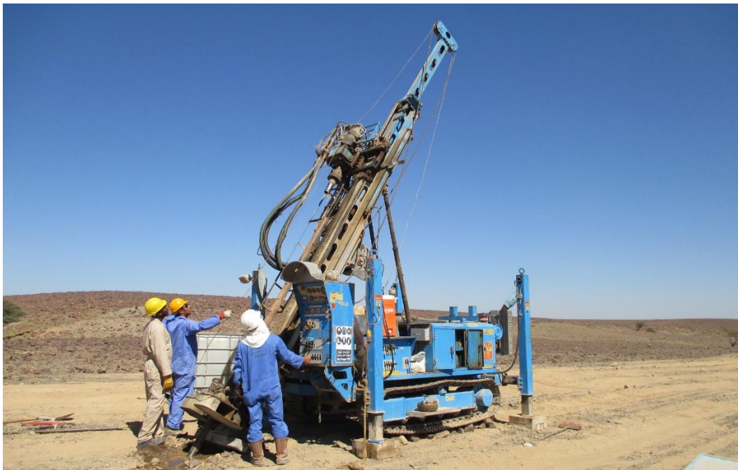
Figure 2: Gulf Geotech diamond drill rig drilling at priority EM target at Sarami West
