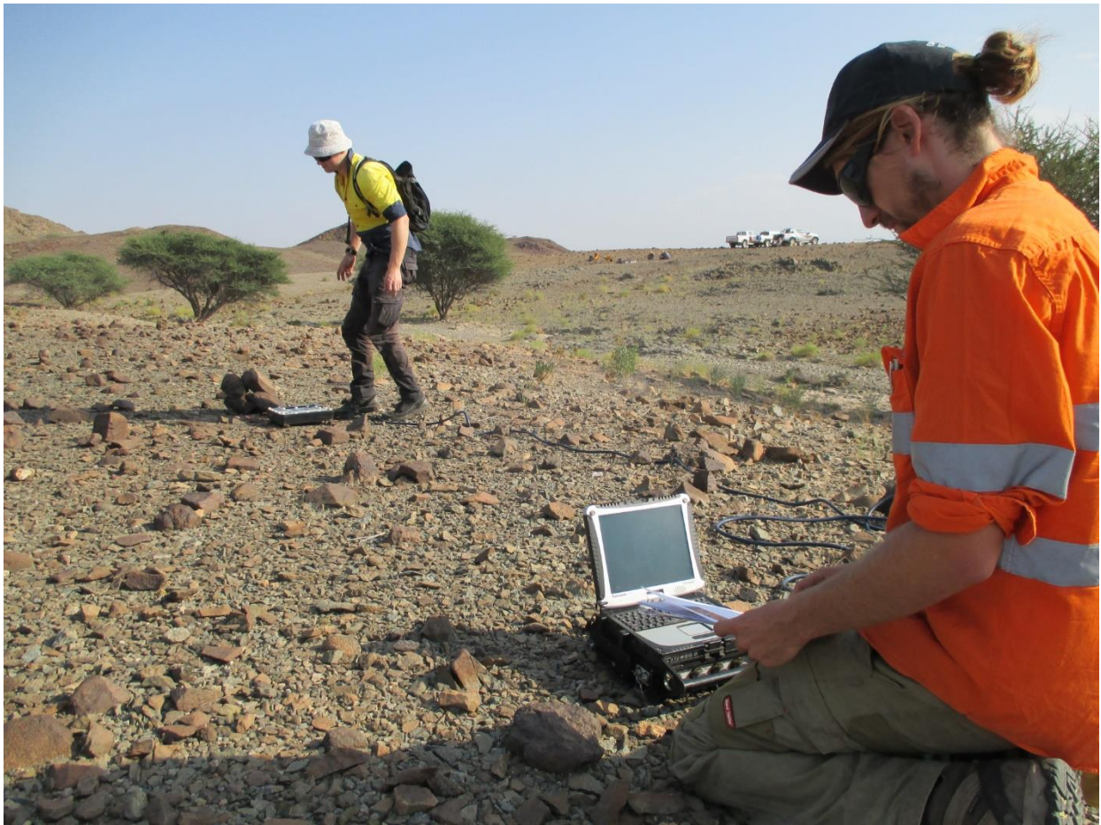
Figure 1. Ground Electromagnetic Survey at Sarami West VTEM Anomalies
