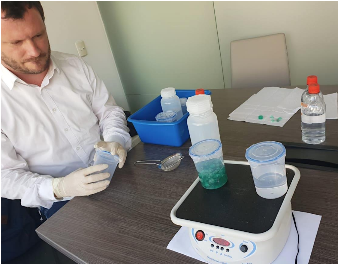
Image 1: Applying the physical tracers to Fura's sample emerald rough from the Coscuez Emerald Mine.
