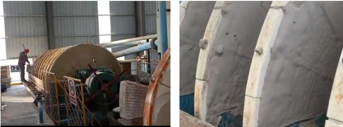
*Figure 2 – Flotation product undergoing filtration for reduction of moisture content to <5%*
