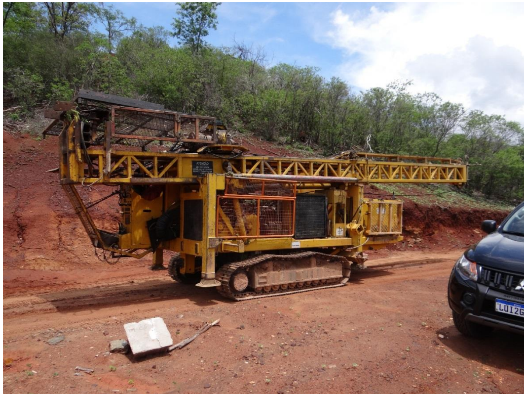
Figure 2 – Drill rig (UDR-200) on site (Pitombeiras North target).
