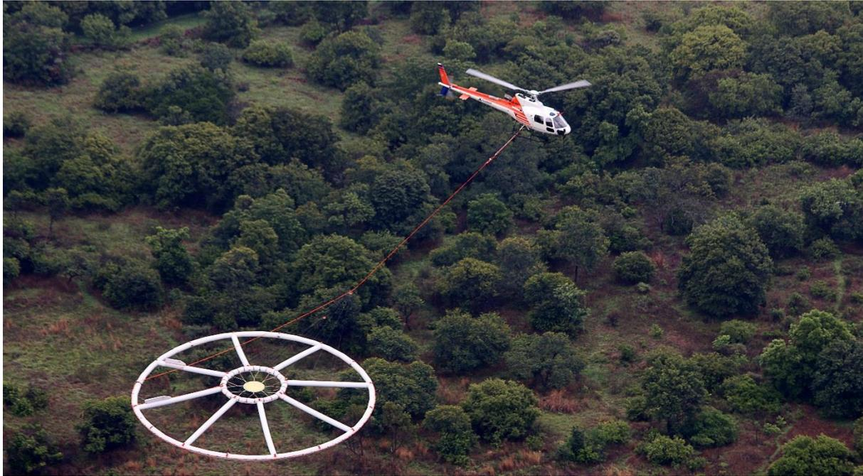
**Figure 4. NRG’s Xcite™ systems are towed arrays, using high performance AS350 B-series helicopters (or similar). The AS350 is ideal for the close terrain following required for geophysical surveys.**
