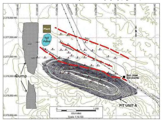
Figure 45. Plan of Proposed Mine Pit, Plant, Dumps and Tailings.
