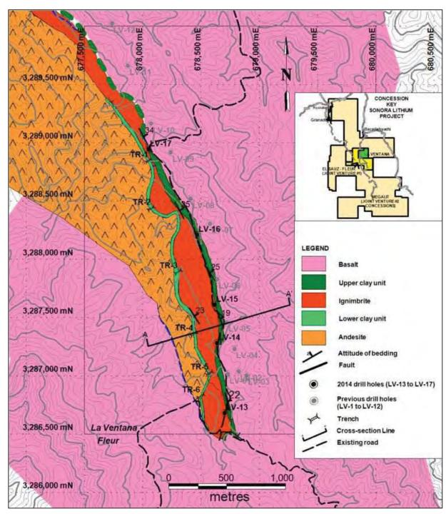
Figure 24. Drill Hole Location Plan La Ventana Concession.
