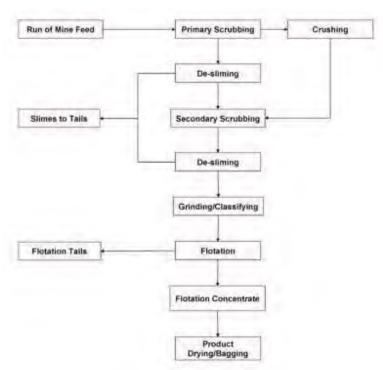
Figure 47. Conceptual Colemanite Process Flow Diagram.
