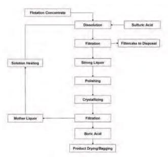
Figure 46. Boric Acid Process Flow Diagram.
