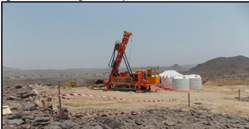
Figure 3. Diamond Drill rig on site at Bayda
