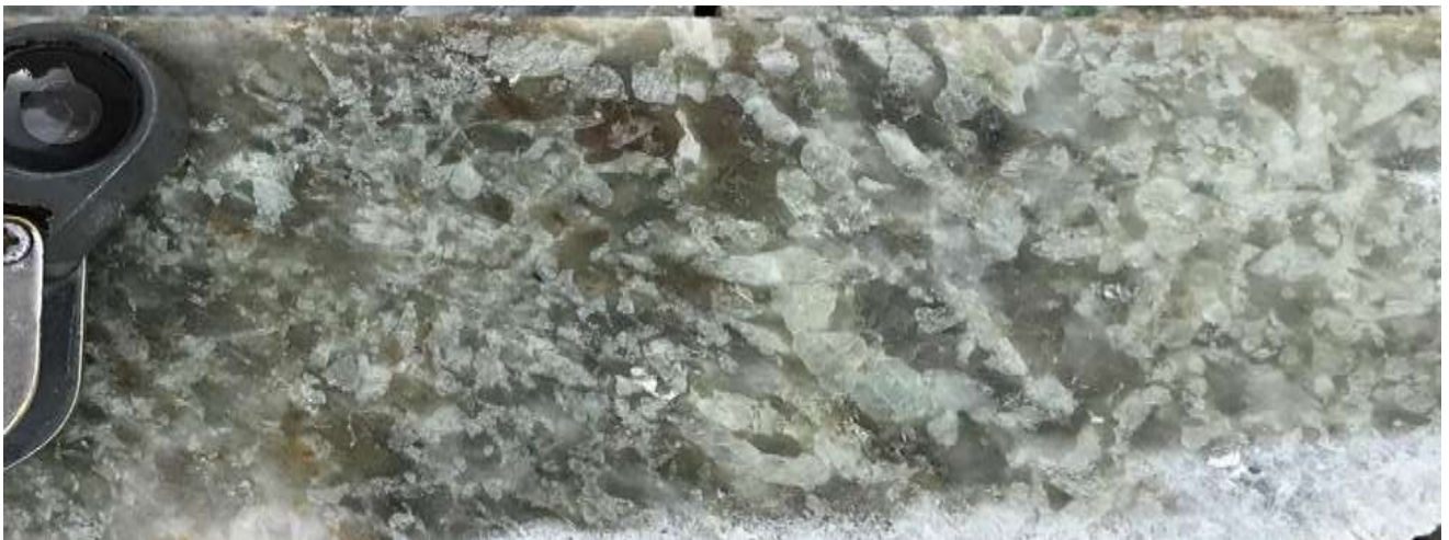
Figure 5: Typical P2 finer grained spodumene (<20mm long crystals) pegmatite in half core (diameter of hand lens approx. 2cm)
