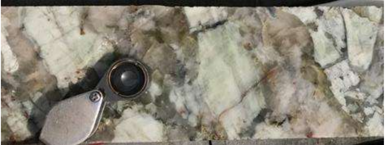
Figure 4: Typical P1 coarse grained spodumene (>20mm long crystals) pegmatite in half core (diameter of hand lens approx. 2cm)
