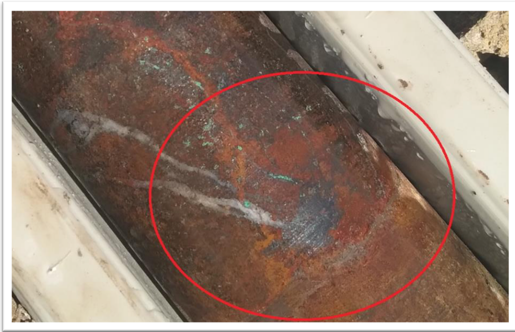
Figure 4: Native silver with associated copper (green) in drill core, drillhole EHDD003, 16.5m depth, Elizabeth Hill, September 2021
