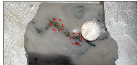
BBDD019: Visible gold identified in pyrite stringer within c. 1m wide quartz-tourmaline vein at 70.90m downhole
