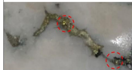
BBDD019: Visible gold identified in pyrite stringer within c. 1m wide quartz-tourmaline vein at 70.90m downhole
