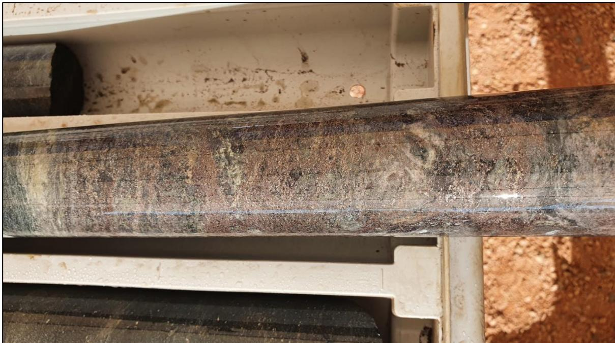
Pyrrhotite mineralisation with the hanging wall basalt above the Bellevue Style quartz veining (194.0m-204.80m shown).
