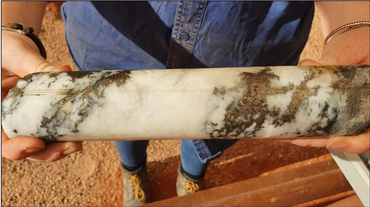
Bellevue Style mineralisation with white quartz hosting sulphide mineralisation KVRD025 (201.5m-202.0m shown).
