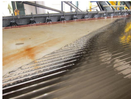
Shaking Table Cleaning 12tph
