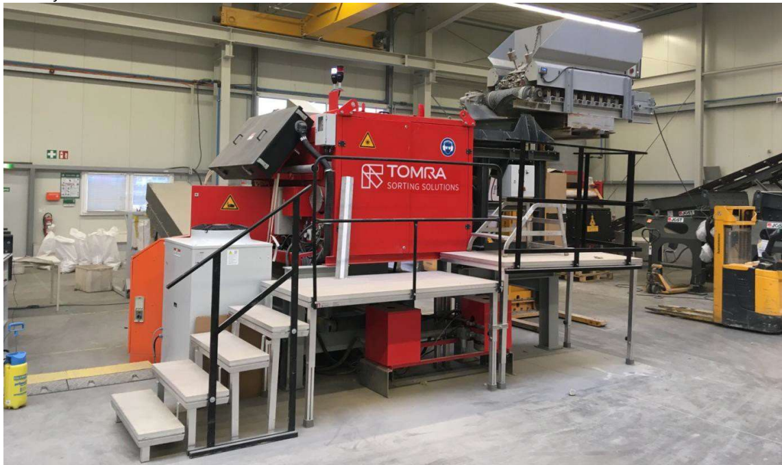
Figure 1: Laser sorter: 3D model of Laser sorter (top) and Laser sorter test rig in Tomra's technical center used for fraction +25 mm
