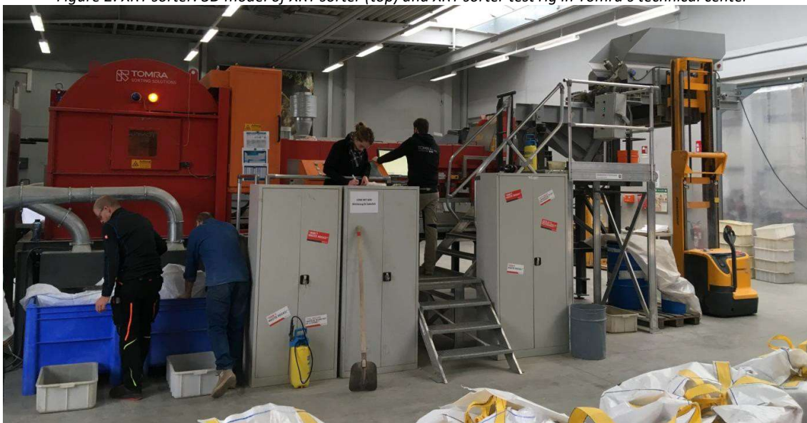
Figure 2: XRT sorter: 3D model of XRT sorter (top) and XRT sorter test rig in Tomra's technical center
