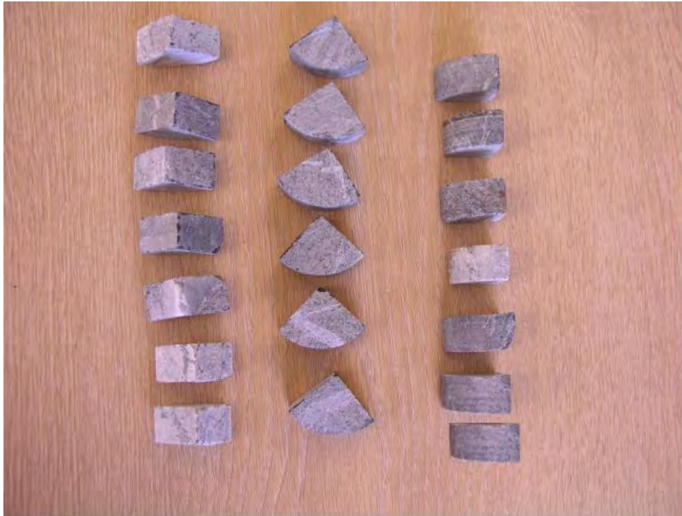
Figure 5 – Orientations of Pieces for Breakage (Cut Core Method)
