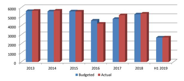
Analysis of the production data shows that the produced gas volumes were almost equal or exceeded the expected gas volume. We may say that the natural decline of the gas reservoirs was mitigated in this period, recording a value of approximately 1.4 % for the period 2013 - 2019.
