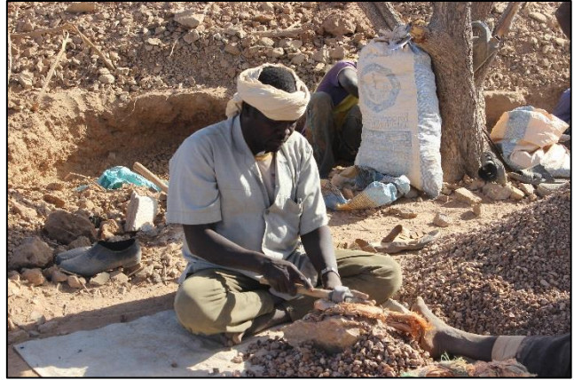
Left: artisanal workings at the Dorothe license. Right: artisanal crushing and visual sorting of high-grade visible gold in quartz vein material.
