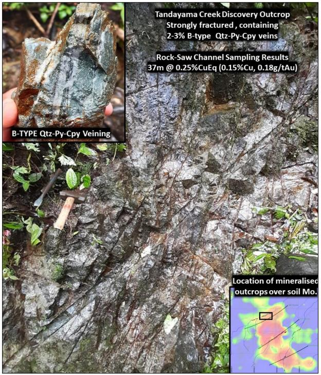
**Figure 7**: Rock-saw channel sampling over surface exposure in Tandayama Creek returned a significant assay result of 37m @ 0.25%CuEq (0.15Cu, 0.18 Au). This work was completed in mid-2016 as part of routine exploration on the tenement where B-type porphyry quartz veins hosting chalcopyrite mineralisation were discovered at surface.
