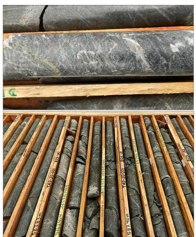
**Figure 4**: Selected drill core example of strong visible chalcopyrite copper sulphide mineralisation within a quartz-diorite intrusion in TAD-20-001. Drill core is HQ size or 63.5mm in diameter.
