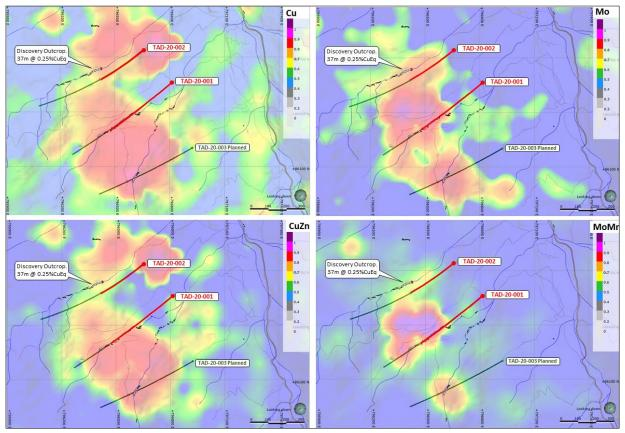
**Figure 6**: The Tandayama-America target is characterised by coincident Cu, Mo, CuZn ratio and MoMn ratio soil geochemical highs centred upon outcropping mineralisation in Tandayama and America creeks.
