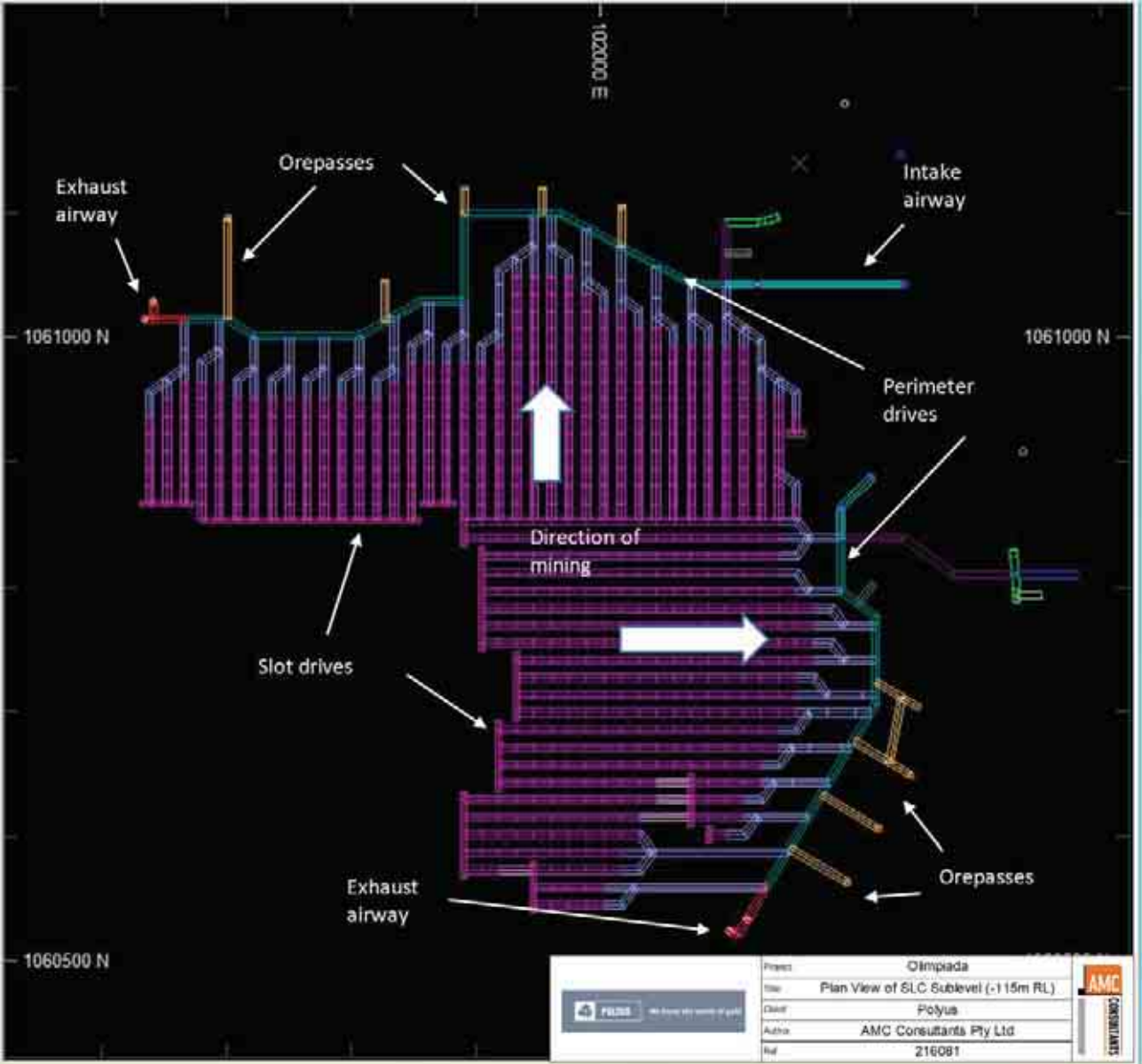
Figure 2.8 Olimpiada - plan view of the layout of an SLC level (-115 mRL)
