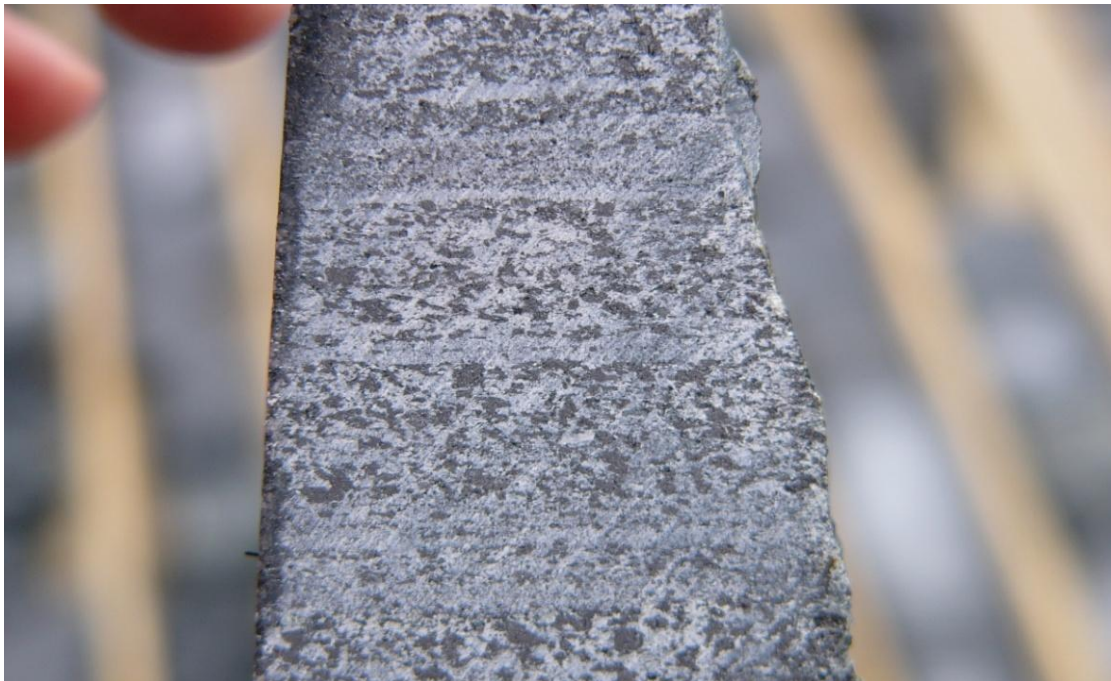
Figure 2-1: Hand specimen of Havik East coarse magnetite (Source: SRK)
