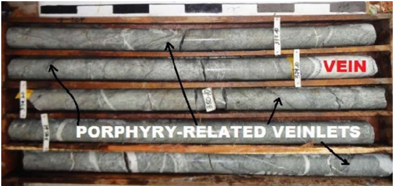
Photo 3. Chloritic altered andesite porphyry intrusive with porphyry-related 2-3mm wide greyish quartz-sulphide veinlets (0.14 to 0.18% Cu & 0.14 to 0.23 g/t Au) overprinted by a 200 mm wide milky epithermal quartz vein (98.76 g/t Au) and other narrower ones. (Hole EXP089: 377.75 to 382.35 metres).
