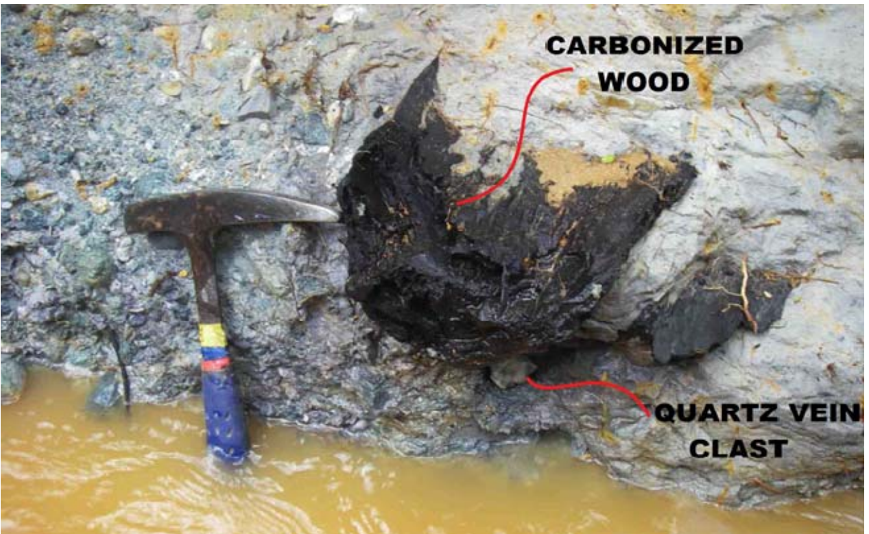
Photo 2. Polymictic conglomerate with carbonised wood and quartz vein clasts.
