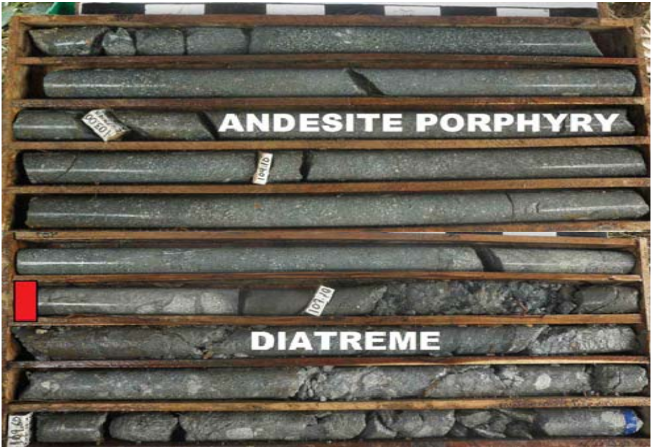
Photo1. Contact of the upper andesite porphyry to diorite megablock with the underlying diatreme (Hole EXP093: 101 to110.55 metres).
