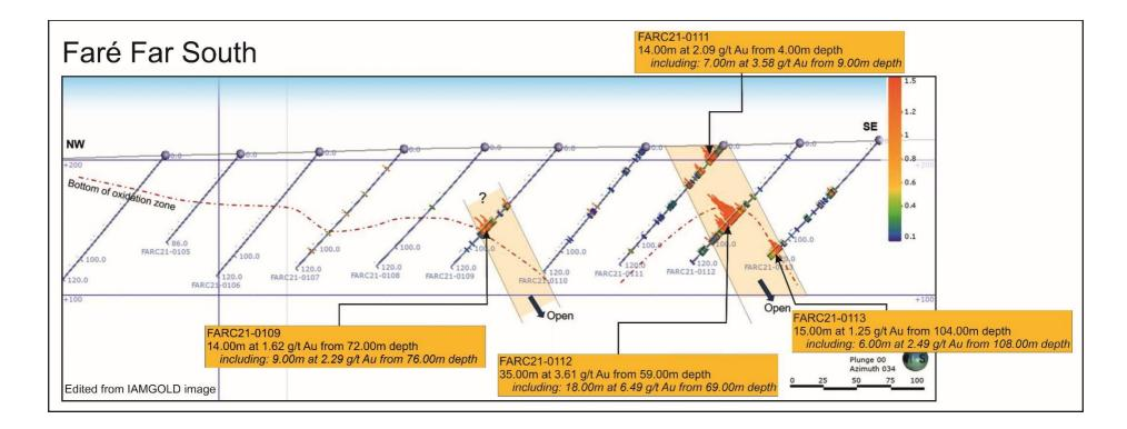
Faré Far South anomaly – 2021 RC drilling cross section for northernmost fence line, including best results to date
