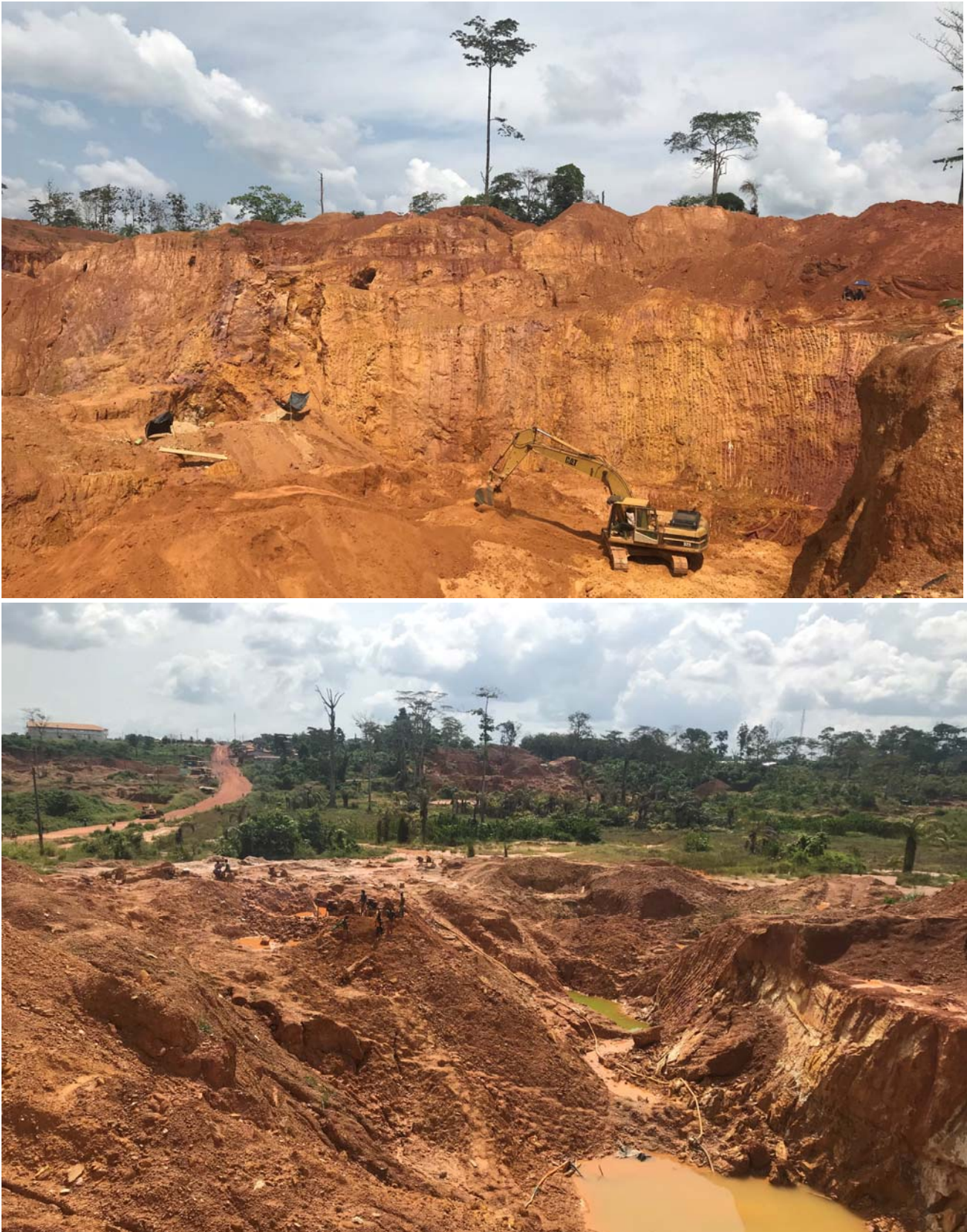
Figure 5 | Large-scale, 'hard-rock' artisanal workings observed within the license area and occurring along a 1.6km strike target zone. Top Photo: taken looking north-east; note sub-vertical structures and iron oxide staining within harder rocky promontory above black tarpaulins with prior underground artisanal shafts and adits visible in the pit wall; excavator for scale. Bottom photo: this artisanal working occurs adjacent to the working in the top photo; note strike extension of artisanal working in opposite stream bank wall suggesting continuity of mineralisation; people for scale
