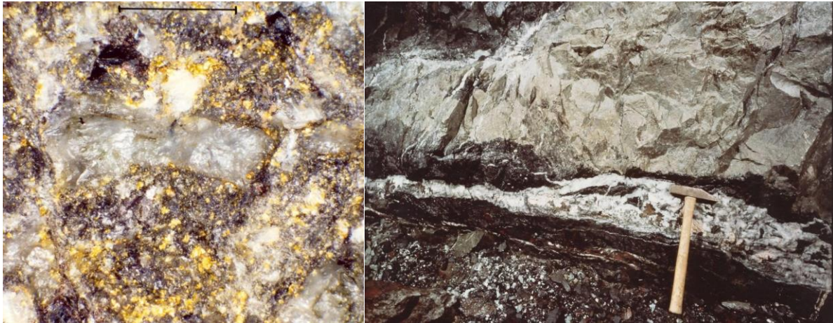
Figure 5 (left): Very high-grade visible gold ore from the footwall leader vein (FLV) within the Chidlaw Link Zone, 40 Level, Gwynfynydd mine. Scale bar 5 mm; (right) FLV from which this material was extracted during a past period of production. [Source: Snowden Mining Industry Consultants Pty Limited Technical Report, 2012]
