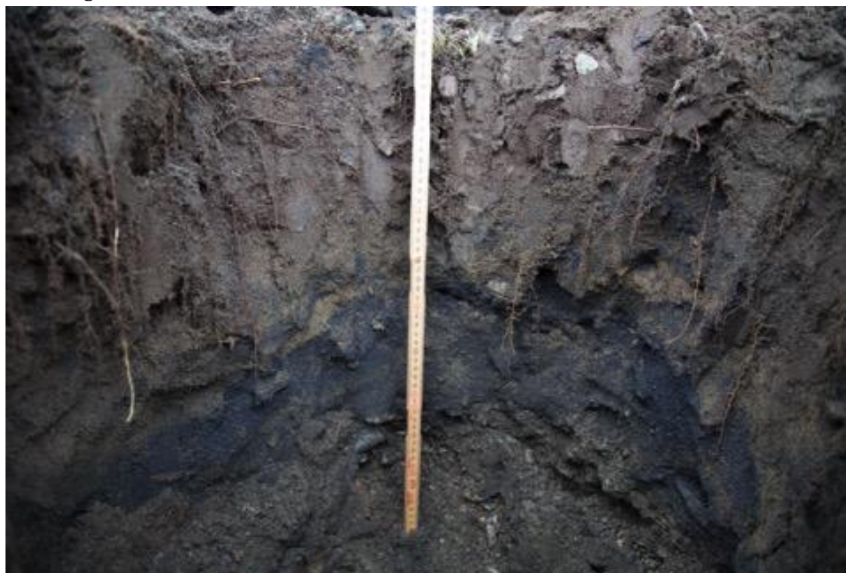
Figure 2. Initial trenching demonstrating ilmenite depositional models. Black banding is almost pure ilmenite; total depth of ilmenite bearing sediments is unknown.
