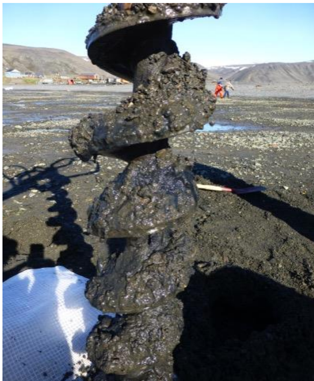
Figure 1: Auger sample from raised beach (black material is ilmenite rich sediments)
