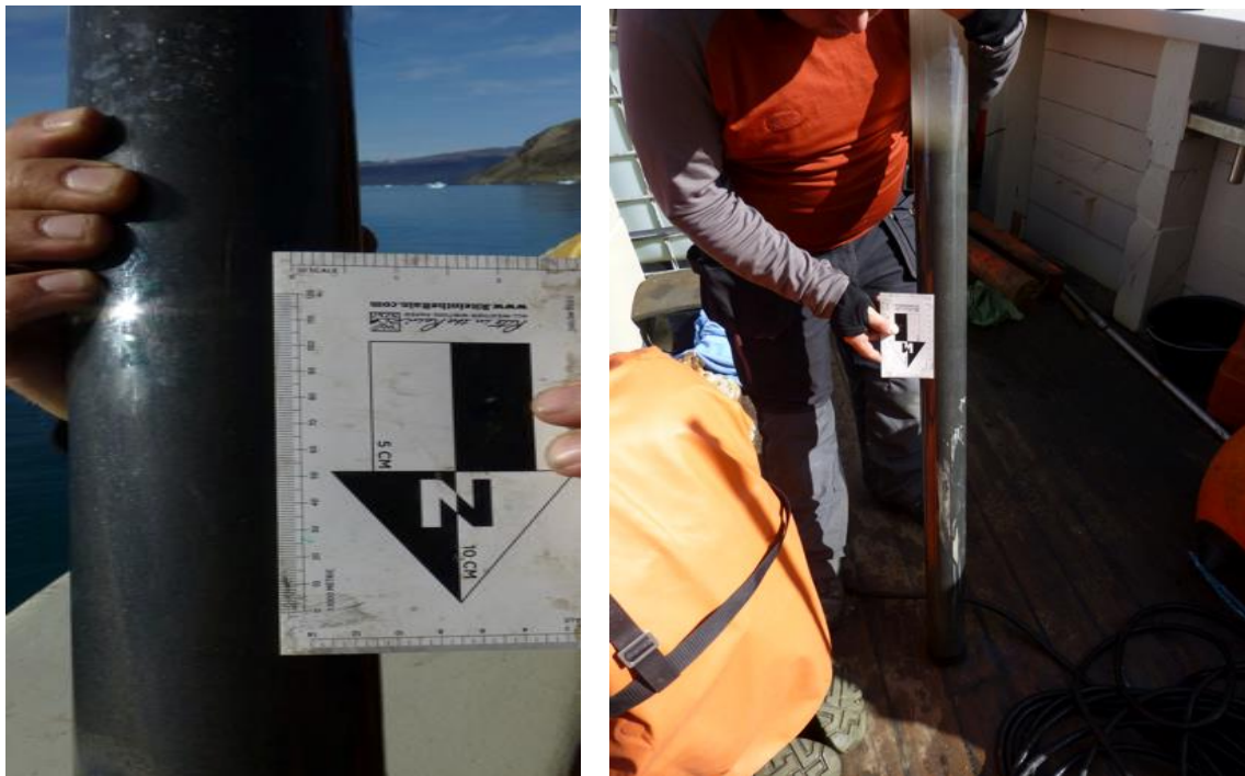
Figures 3 & 4: Ilmenite rich black sand in vibracore stem from Kisaq.
