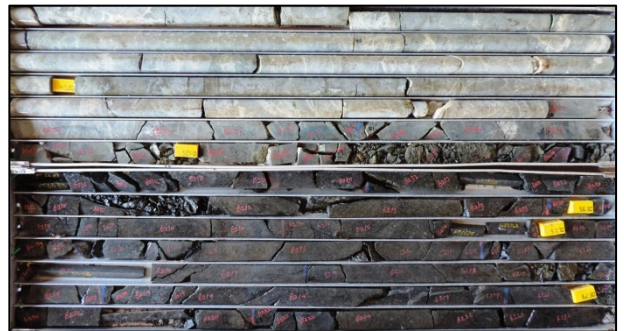
Contact between Transvaal Supergroup metasedimentary hanging wall and Platreef-style intrusive in drill hole 2022.
