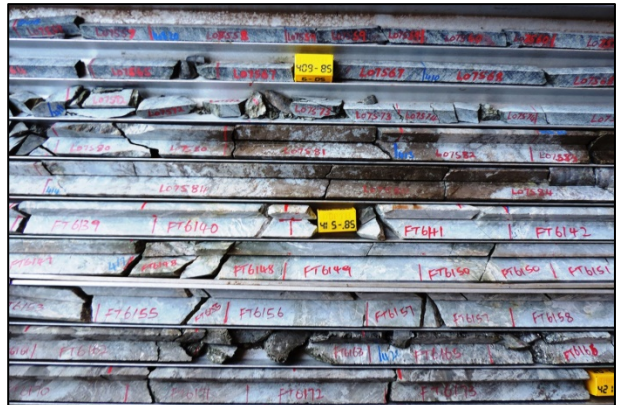
Massive sulphide zone towards the base of drill hole Z017.
