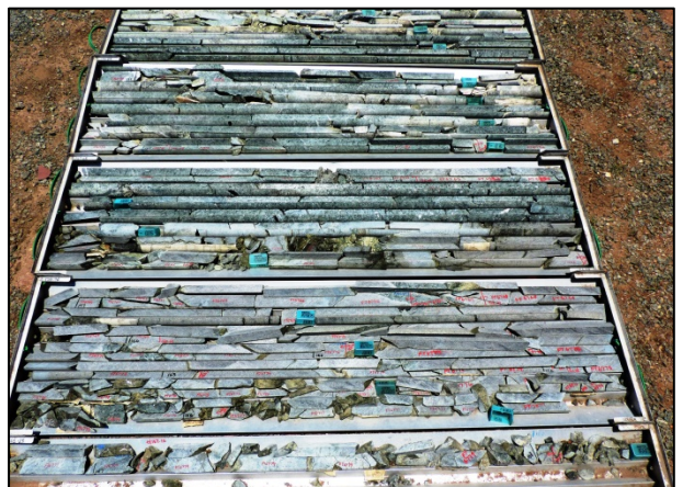
Drill hole Z01 showing faulted contact between serpentinized dunite and Platreef-style feldspathic pyroxenite.
