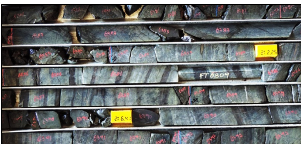
Drill hole 2020: magnetite layers in the footwall Transvaal Supergroup metasedimentary strata.
