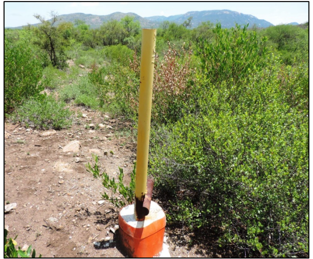
Collar stand pipe for drill hole Z017.
