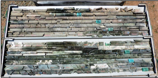
Transvaal - Lower Zone contact zone in drill hole Z01.
