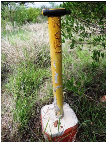
Collar stand pipe for drill hole Z021.
