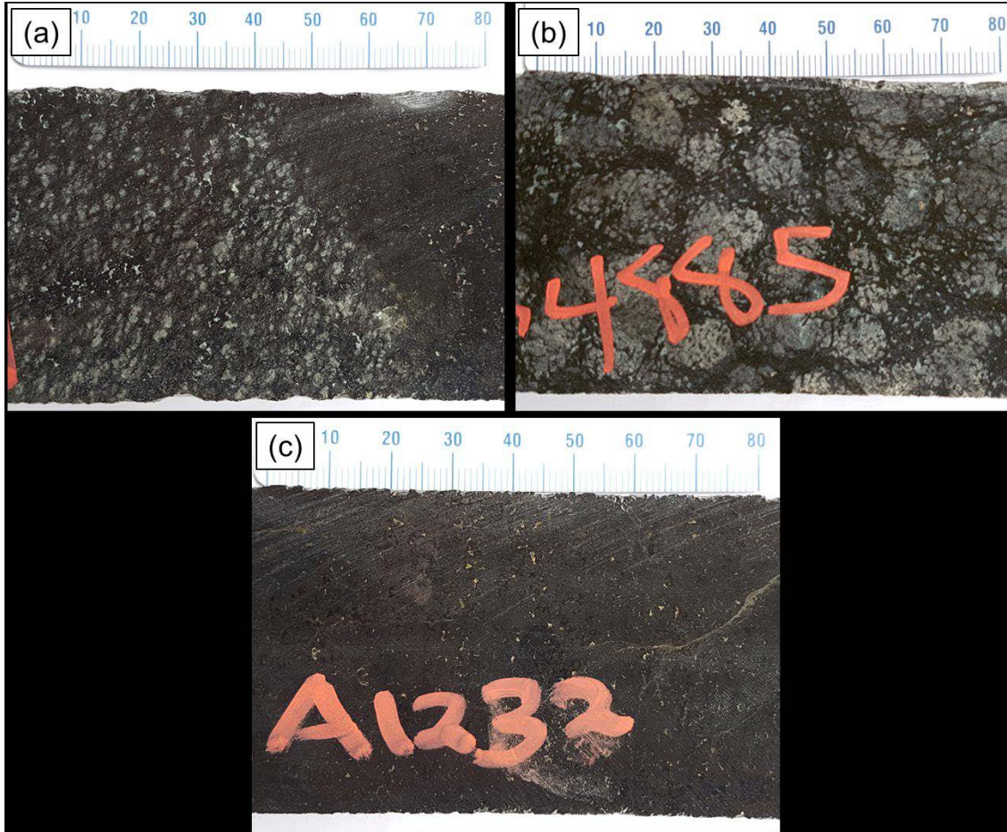
Figure 7-8: Main lithologies seen in the Lower Zone Uitloop II body: (a) medium-grained serpentinized dunite, (b) poikilitic harzburgite, (c) fine- to medium-grained serpentinite with finely disseminated pyrrhotite and pentlandite sulphides (McCreesh et al. , 2019).
