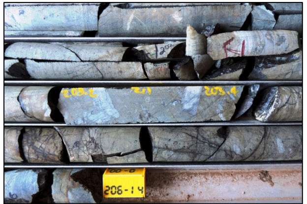
Dolomite xenoliths at the base of drill hole 2019.
