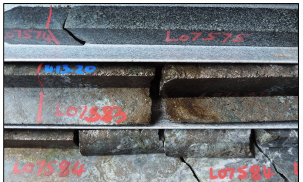
Drill hole Z017 - Lower Zone metasedimentary contact with massive and blebby sulphides.
