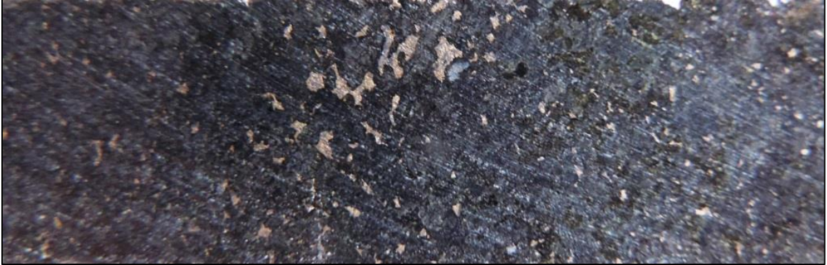
Figure 7-13: Bleb sulphides in drill hole Z022 from the Platreef/Critical Zone.
