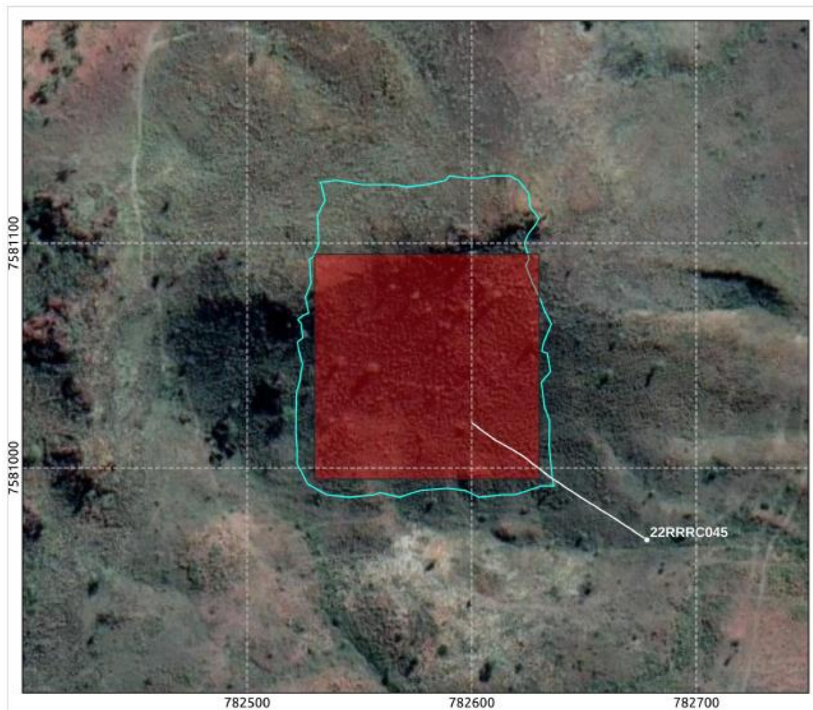
Figure 3: EM conductor identified by FLEM survey and location of RC drill hole trace overlain on the airphoto.
