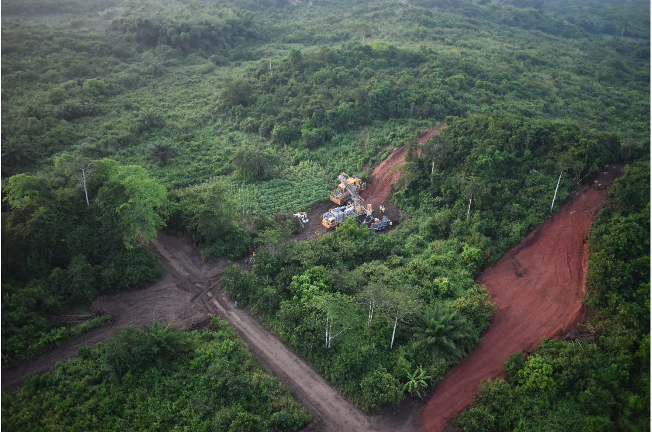
Figure 1 | Aerial view of RC drill rig and support vehicles drilling at one of the Abonko targets with spodumene bearing pegmatite boulders visible on the adjacent drill pad along the topographic high on the right-hand side of the photo
