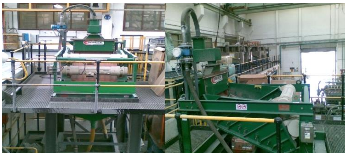
Figure 1 – Pilot scale Derrick Stack Sizer circuit used in beneficiation pilot program at Mintek.
