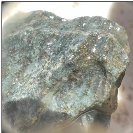
Figure 11: RC drill chip (~3cm in diameter) ARC396 [107-108m] 1% pyrite and pyrrhotite in silicified sericite matrix. Assays are still pending for this hole.
