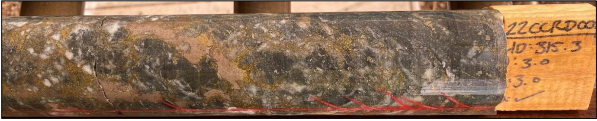
Figure 7: ~300mm of HQ drill core - 22CCRD008 mineralisation occurrence at EOH 315.3m.
