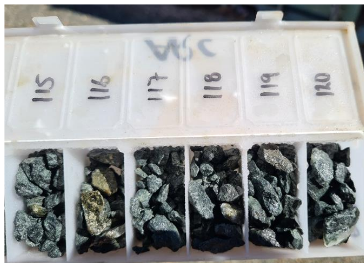
Figure 14: RC drill chips - Sulphide occurrence in ARC403 comprising pyrite and pyrrhotite. Assays results are pending. Each chip compartment is 25mm wide.
