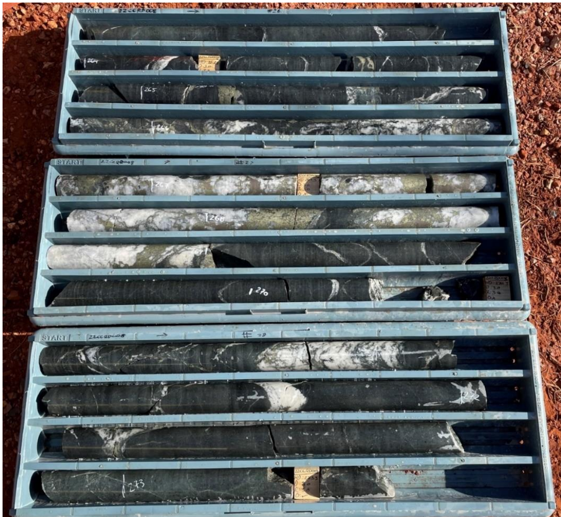
Figure 6: HQ drill core - 22CCR008 (263-273.5m) interval of significant vein hosted sulphide forming lower part of the broader 16.6m interval with a significant grade of 3.14m @ 6.38% Cu, 3.61g/t Au, 0.059% Co from 265.92m. Core tray is 1065mm long.
