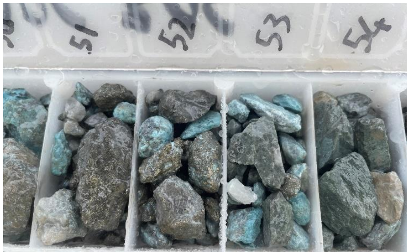
Figure 9: RC drill chips - Interval of sulphide and fuchsite(?) in Hole ARC395. Assay results are pending for this hole. Each chip compartment is 25mm wide.
