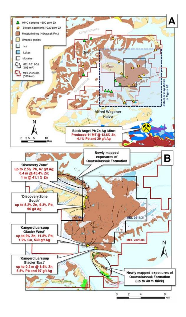
**Figure 1. (A)** Geological map showing Bluejay's Kangerluarsuk Zinc-Lead-Silver Project, comprising of the Mineral Exploration Licences 2011/32 and 2020/06; **Figure 1.(B)** Geological map showing the positions of newly mapped exposures of Qaarsukassak Formation (host to the known Zn-Pb-Ag mineralisation within the licence areas). Results of sampling by RTZ in the early 1990s also shown for mineralised showings
