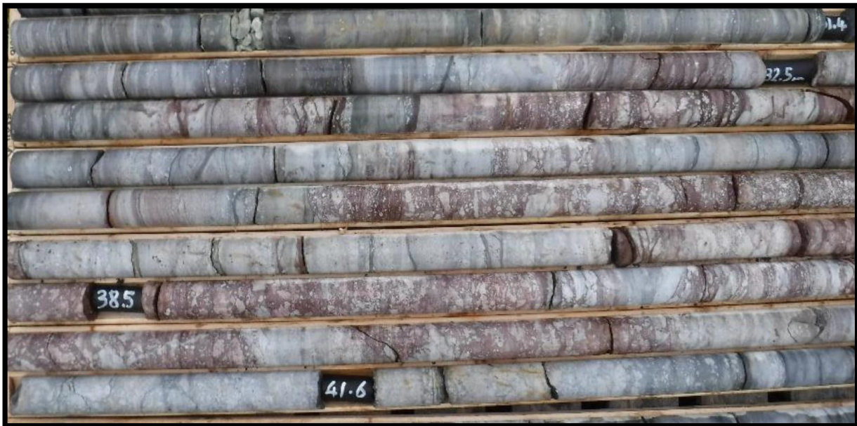
Figure 2: Debris flow or fault breccia with haematitic matrix in drill hole 19-3824-02
