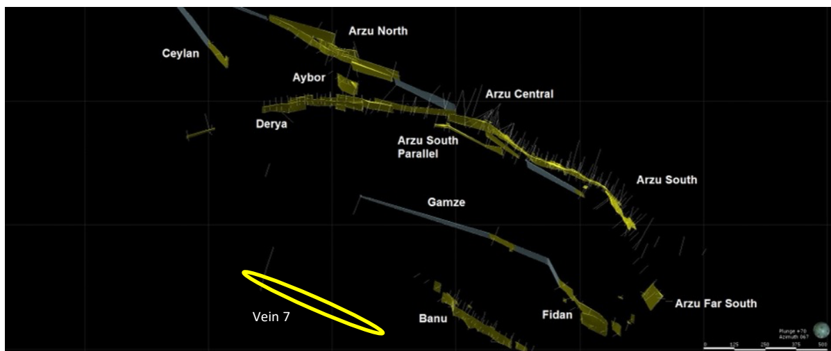
Figure 3: Three-dimensional model of the Kiziltepe vein system, with Banu shown towards the bottom of the frame. The Vein 7 area lies adjacent to Banu and is highlighted.
