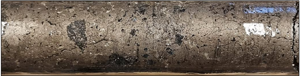
Figure 1: Massive pyrrhotite-pentlandite-chalcopyrite with coarse grained pentlandite and rounded clasts of peridotite, from a 0.3 m sample that returned 2.23% Ni, 0.15% Cu, 0.20% Co, 176.83 m, 23RAN002. NQ diameter drill core.
