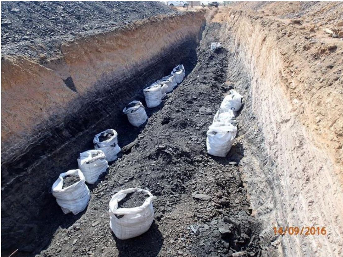
Pit 2 sampling showing coal seam 2.5m thick at 3 metres below surface
