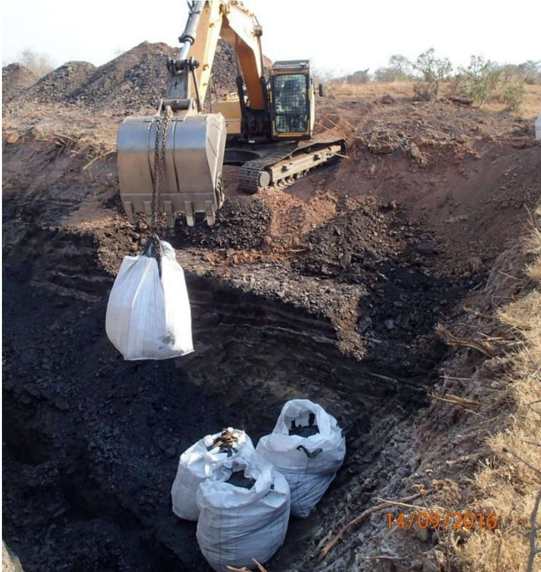
Pit 1 sampling showing seam 2,4 metres below surface
