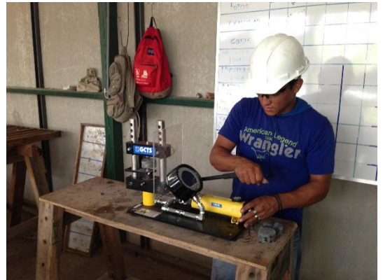
Figure 11. Point load testing geotechnical drill core samples.
