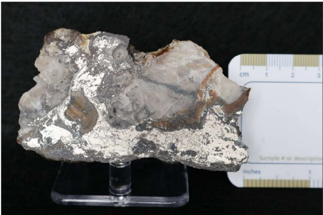
Figure 1. Photograph of polished sample showing high-grade, native silver mineralisation in a carbonate vein. Sample taken from the Elizabeth Hill mine site. The sample is visually estimated to host ~10% silver (~100,000 g/t). Visual estimates are approximate and are only suggestive of local specimen grade and not the mineralized deposit as a whole.
