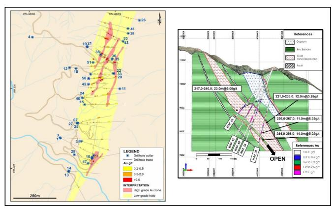
Figure 3. APTA Drill Plan and Section
