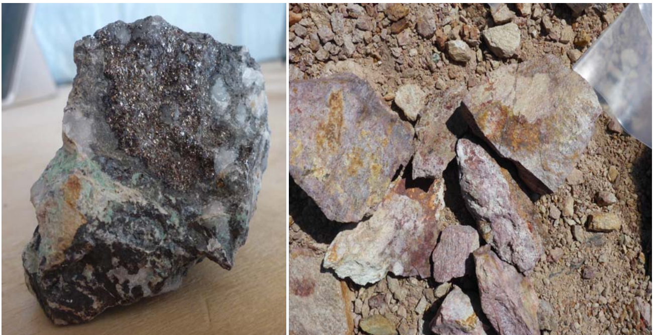
Figure 1 | High-grade vein material at 39.1g/t Au, 789g/t Ag, >20% Pb and 0.48% Cu from new artisanal workings within the Dorothe prospect (left) and host wall-rock alteration grading up to 1.27g/t Au, 8.1g/t Ag, 1840ppm Pb, 274ppm Cu (right)
