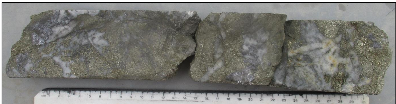
Figure 2: Split section of drill core from hole FR-DD-22-UG-186 grading 110.1 g/t Au and 115 g/t Ag over an estimated true width of 0.21 metre.
