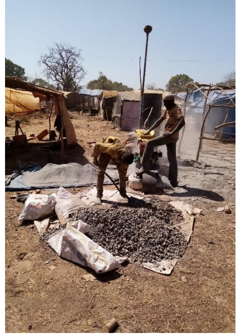
Figure 5: Semi-mechanised Crushing of Hard Host Rock (note lack of quartz)
