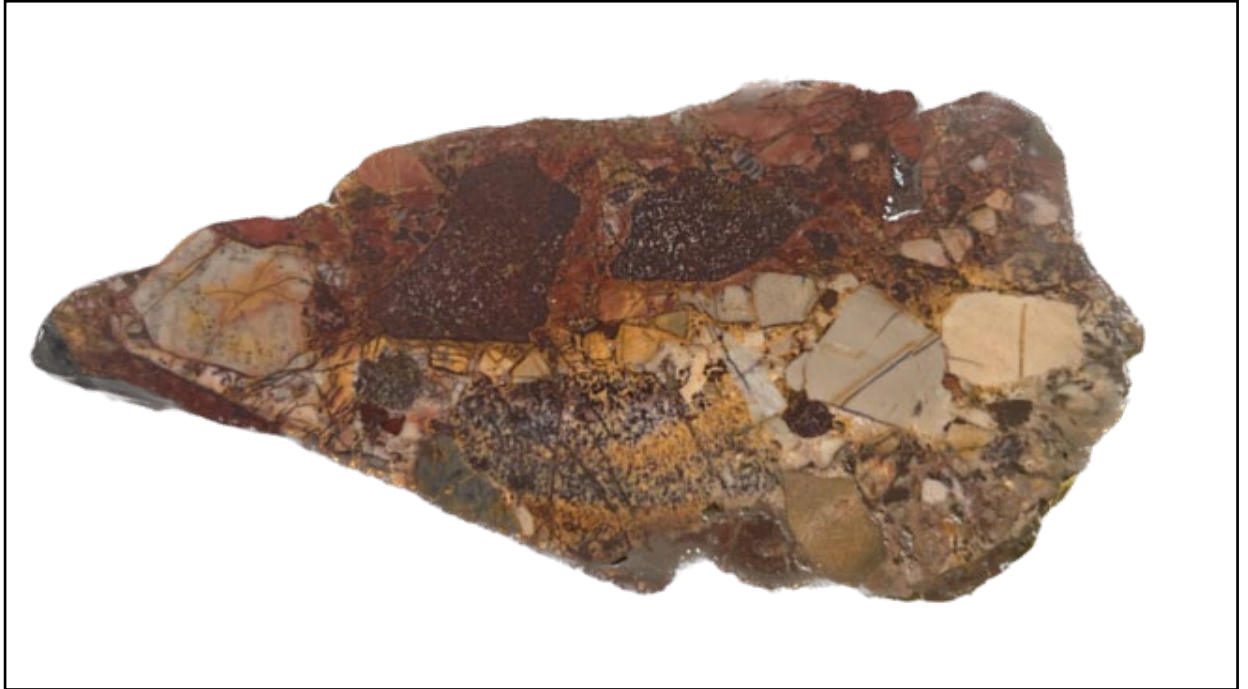
Figure 2: Sample of polymictic breccia from the mineralised southern margin of the Plateau rhyolite (PL23_002).
