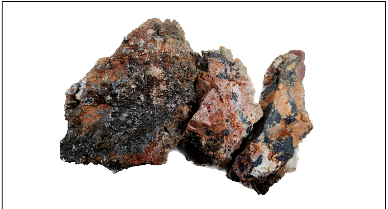
Figure 4: Sample of manganiferous gossan from Cardigan Dam that is elevated in gold, silver, copper, cobalt and barium.
