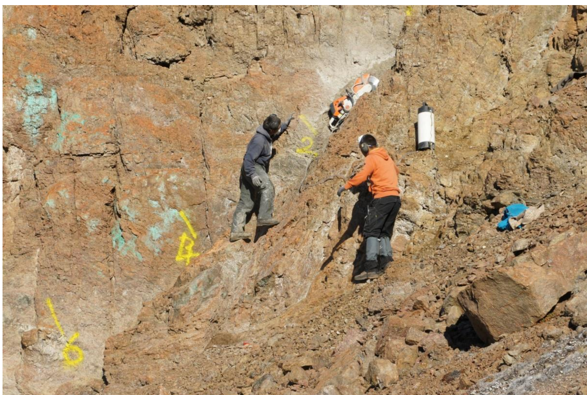
Figure 2: Historic Martome prospect sampling showing evidence of copper mineralisation (green staining)
