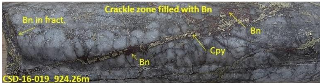
Image 1: Bornite-rich mineralisation characteristic of shallower portions of the known deposit at Alpala, here exemplified in Hole 19.
