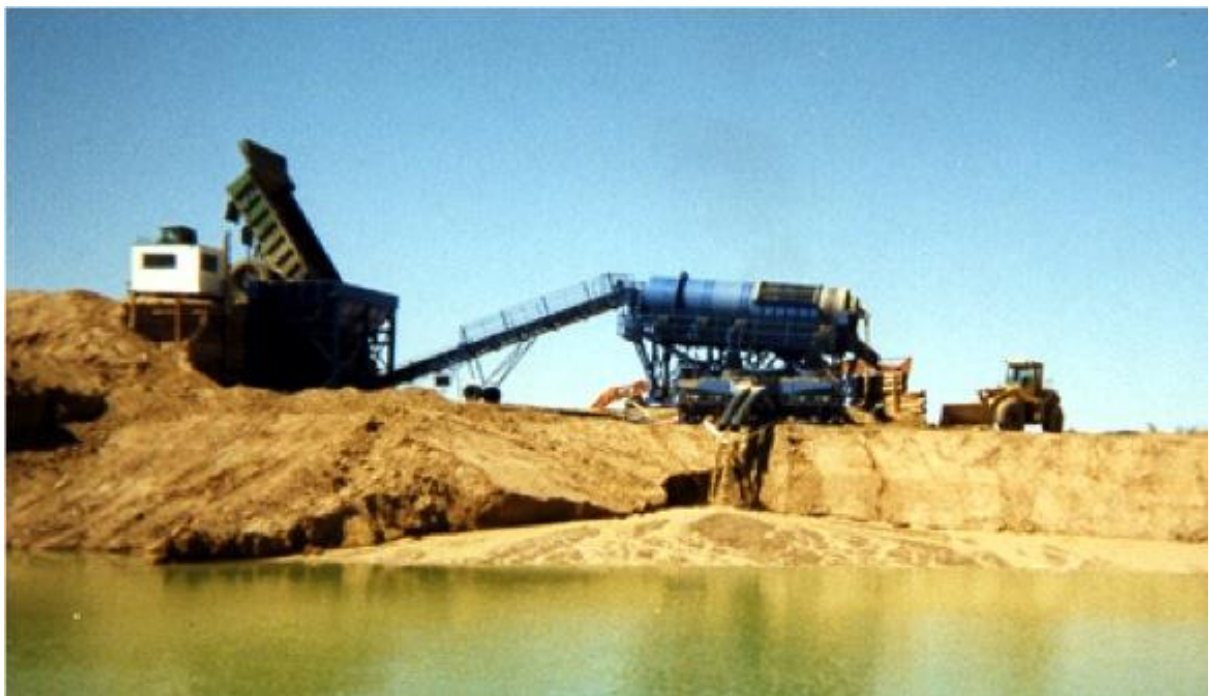
Figure 3. 200 LCM per hour processing plant at Nardoo
